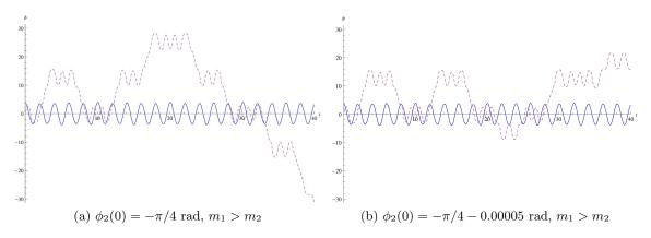
Figure 2:  $\phi_1$  and  $\phi_2$  (dashed line) as a function of time; the initial values in (a) (b) are identical except for a small variation in  $\phi_2(0)$ .
