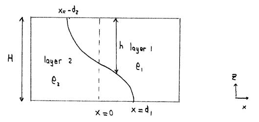
At time t = 0 the vertical wall is removed and the system adjusts to a final steady state. In the figure, the interface between the two fluids in the end state is indicated by the solid curve (from  $x = -d_2$  to  $x = d_1$ ). Note that thickness h = H - a. The dynamics is governed by the nonlinear, frictionless shallow water equations for a two-layer system on the f-plane.
