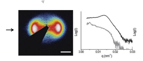
Above you see the 2D scattering pattern of an aligned liquid crystal phase and two intensity line profiles. Left: Log of the scattered x-ray intensity versus scattering vector q, the white bar has a length of 0.01 nm<sup>-1</sup> (note the black 'shadow' is the beam stop). Right: Averaged intensities taken in the direction of the two arrows left.
