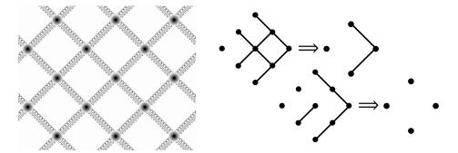
The probability of there being a whole spring (a connection) is p, while the probability of the spring being broken is 1 - p. We consider rupture along the y-axis.
