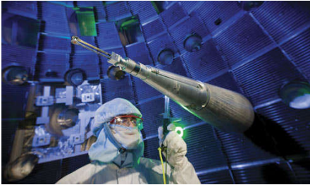
Figure 3: The target chamber of the NIF. In comparison with the huge lasers, the target positioner is (almost ridiculously) small.
